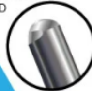
1/2" BOWL GOUGE MICRO-BEVEL GRIND
